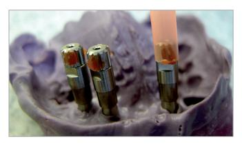
Attach an extension tube (straw, etc.) and seal the thumbscrew with wax to prevent the ingress of plaster in the area between sleeve and screw.
